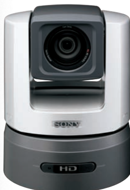
Compact as it is, Sony's PCSA-CHG90 camera achieves exceptional performance with three Sony interline transfer CCDs and a Carl Zeiss Vario-Sonnar lens with T* anti-glare coatings.
